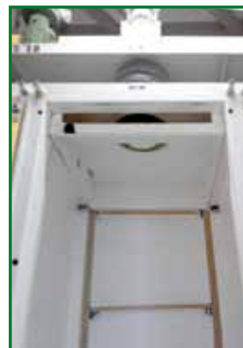
Transformation Plansifter with increased sieving from 290T / 24 to 390 T / 24 h.
