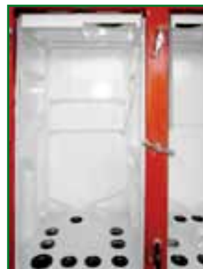
Plansifter transformed with sifting surface increased by 40%
